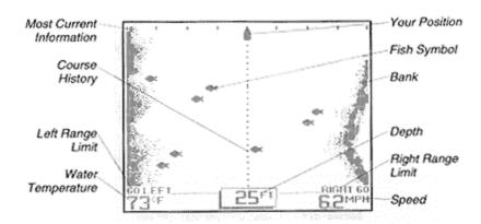
When you exit the "System Options" menu, the view you will see on-screen is shown above. Viewing both left and right sides simultaneously gives you an excellent tool when searching for bait fish or following a creek bed, however greater display resolution can be achieved by viewing only one side.
